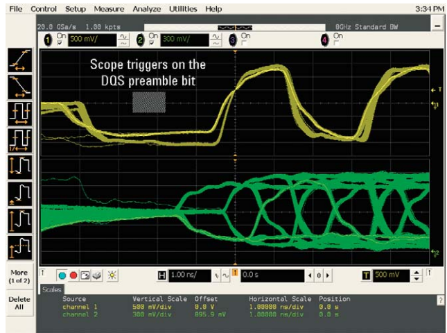
Figure 8. With the “Must Not Intersect” zone drawn, the scope consistently tracks the preamble bits of the read and write signals.
