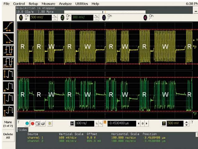
Figure 4. Separating the read and write signals based on the signal amplitude. In this case, you can only separate the read signal because the read signal amplitude is slightly higher than the write signal.
