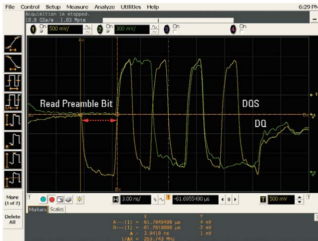
Figure 2. Trigger on the preamble bit of the DQS-read signal
