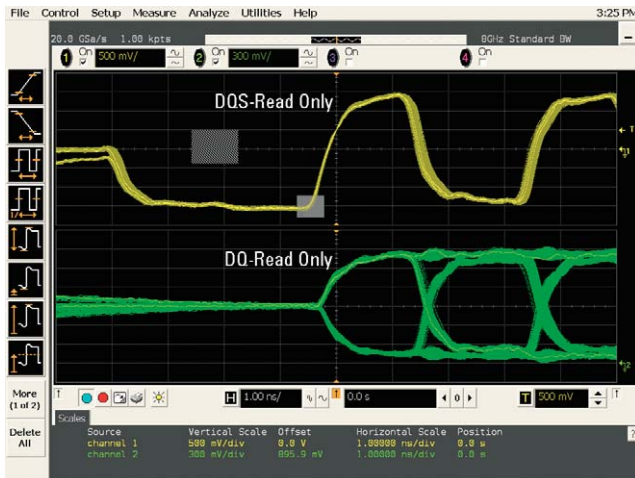
Figure 9. Draw a “Must Intersect” zone at the lower waveform at the preamble bit to track the read only signals.
